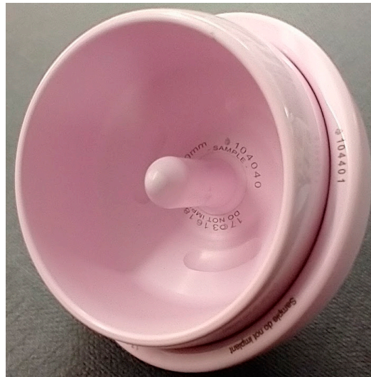
Figure 1. A ReCerf ceramic-on-ceramic resurfacing with modification to the fixation surface for the purpose of experimental simulation.
